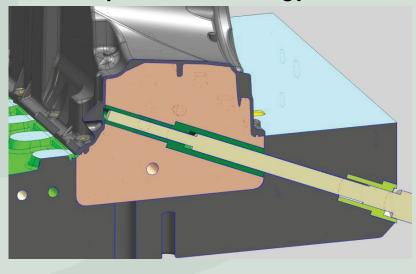
Partial Squeeze technology helps to reduce shrinkage porosity.
