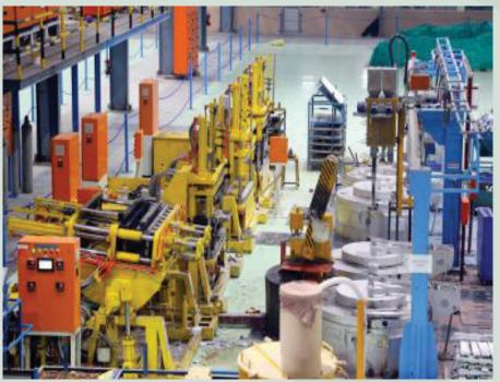
Installed Capacity : More than 5,500 MT / Year GDC With ROBOT – 03 Nos. GDC With Auto Pourer – 04 Nos. GDC With Manual Pourer – 28 Nos. Sand Core Making Machines – 28 Nos. HPDC
